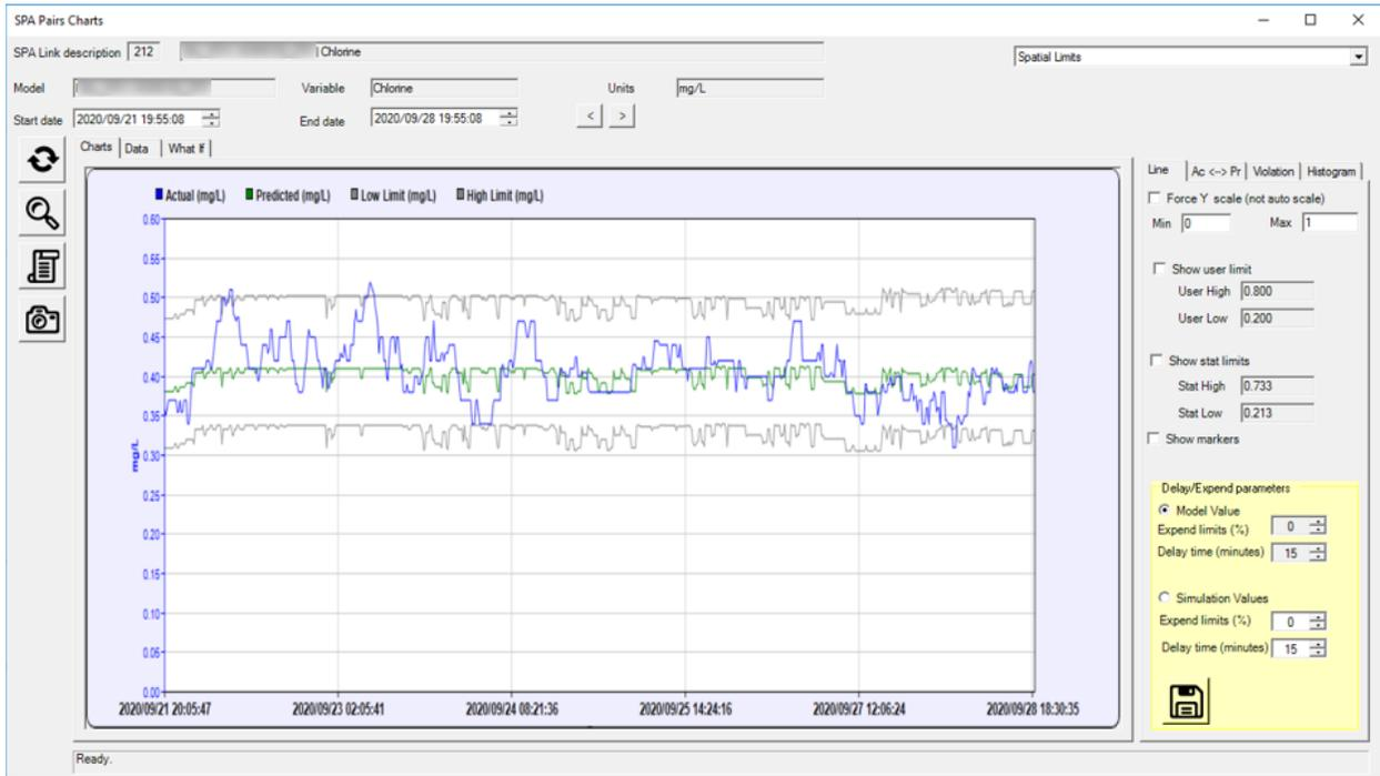
Figure 99: The SPA pairs chart window show the actual, predicted and limit values for the target node in a pair model, as a time series.
