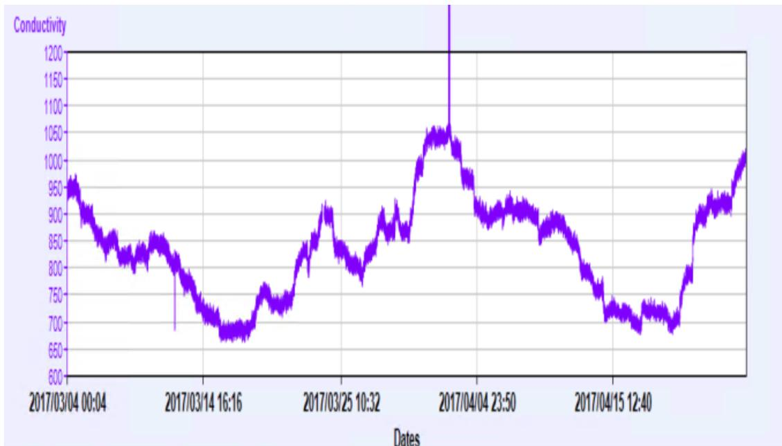
Figure 7: Conductivity measurements for a time period of 40 days in a Source station. Water from this station flows to the station described in Figure 8 (the Target station).
